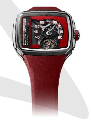
movement developed by HAUTLENCE in 2004: the calibre HL. The small pointer on its end indicates the hour on the vertical scale. Once the 12 numeral is passed, the snail disengages the probe to release the accumulated energy. The linkage then jumps and returns to the 1 numeral. In addition to the linear retrograde jumping hour, the Linear Series 3 is equipped with a flying tourbillon at 6 o'clock, whose balletic movement can be admired behind its black skeletonised bridge.
